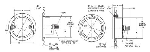
63/100mm Back Connection (XRF) Front Flange Retrofit
